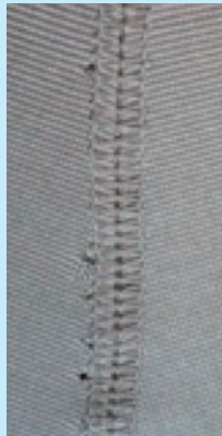
Fabric Yarn Breakage (left side of seam)
