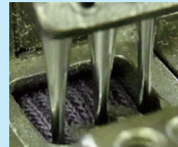
Left needle: KK series Center and right needle: Regular needle
